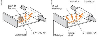
Tests have shown that a very low insulation-fault current (a few mA) can develop and, starting at 300 mA, cause the start of a fire in an environment of damp dust.
