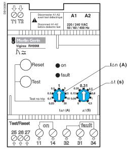
*I*∆*n* (*A*): residual operating-current setting (the relay operates for a fault current ≥ I∆n).
