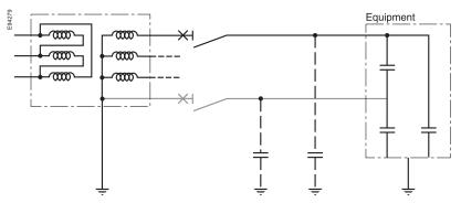
Capacitances between live conductors and earth.
