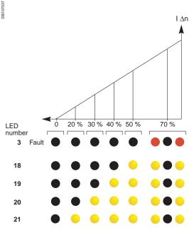
Status of the indication LEDs according to the measured fault current (% I∆n).
