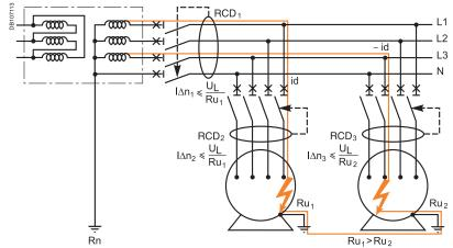
Multiple earth electrodes and flow of current.
