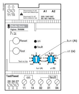
$I_{\Delta n}$  (A): residual operating-current setting (the relay operates for a fault current  $\ge I_{\Delta n}$ ). Schneider Electric guarantees non-operation for all fault currents < 0.8  $I_{\Delta n}$ .
