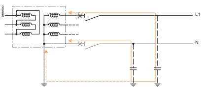
Continuous leakage current due to stray capacitances of conductors (dotted lines).
