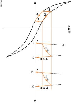
Toroid hysterisis cycle for type A measurements. Id: primary current Im = Id - Ih
