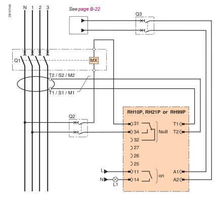
Note: for the RH99 earth leakage monitor use the "fault" contact 31, 32, 34.
