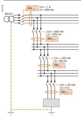
It is possible to divide the installation into a number of groups of circuits and to protect each group using the suitable residual-current device.
