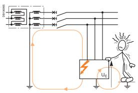
■ Indirect contact: contact of a person with exposed conductive parts that are normally not live, but may become live by accident. This situation is due to failure of the insulation for a device or conductor, resulting in an insulation fault. The electrical risk depends on the touch voltage between the exposed conductive parts of the faulty equipment and earth or other exposed conductive parts located nearby.
