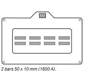
Frame 470 x 160 mm Busbars with 115 mm spacing
