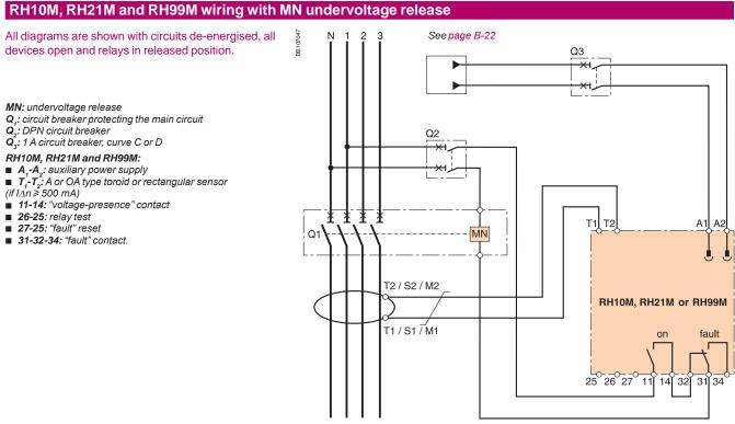
*Note:* for the RH99 earth leakage monitor use the "fault" contact **31, 32, 34**.
