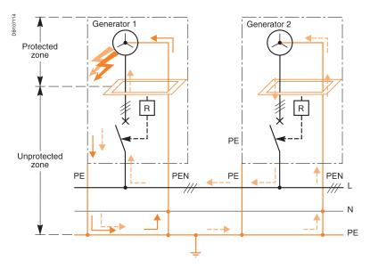
An RCD installed on the generator circuit is the means to:
