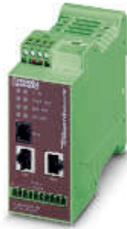
Akıllı Firewall, VPN ve analog modemli router
