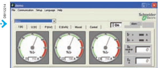
RCU mini-supervision screen for current measurements.
