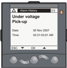
Alarm pick-up and drop-out.
